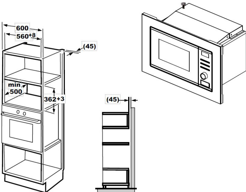
**B. Instalirajte pećnicu**
