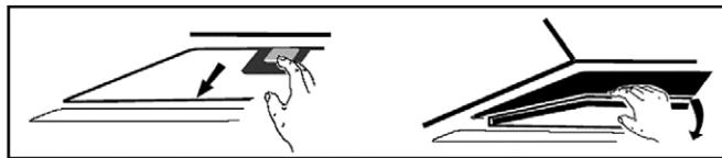
Plug the activated carbon filter into the unit and turn it in clockwise direction. Repeat the same on the other side.
