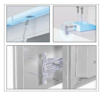
During installation, there is no need to use a ruler, pencil, or similar tools for installing the refrigerator in the cabinet and attaching the door. The installation of the refrigerator in the kitchen unit and door mounting is quick, precise, and simple with the help of stoppers that are an integral part of the refrigerator's brackets and feet.
